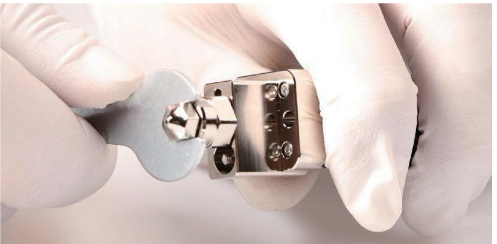
10. Finally, install the silicone sock on the heatblock.
