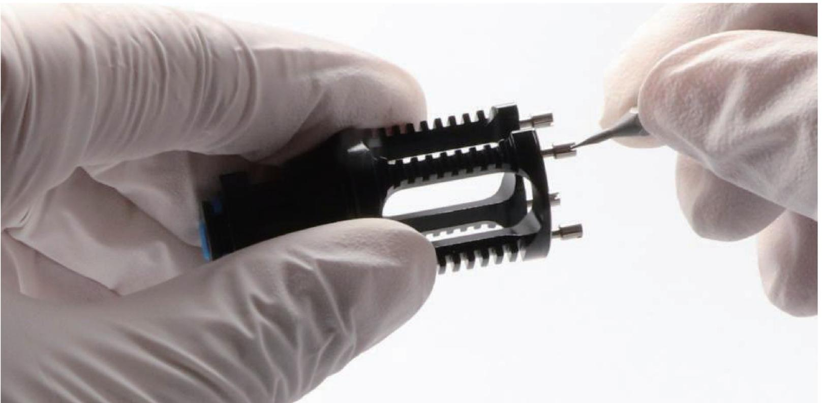
5. Insert the bowden collect into the top of the Adapter, then insert the collect clip between the bowden collect and the Adapter to fix the bowden collect.
