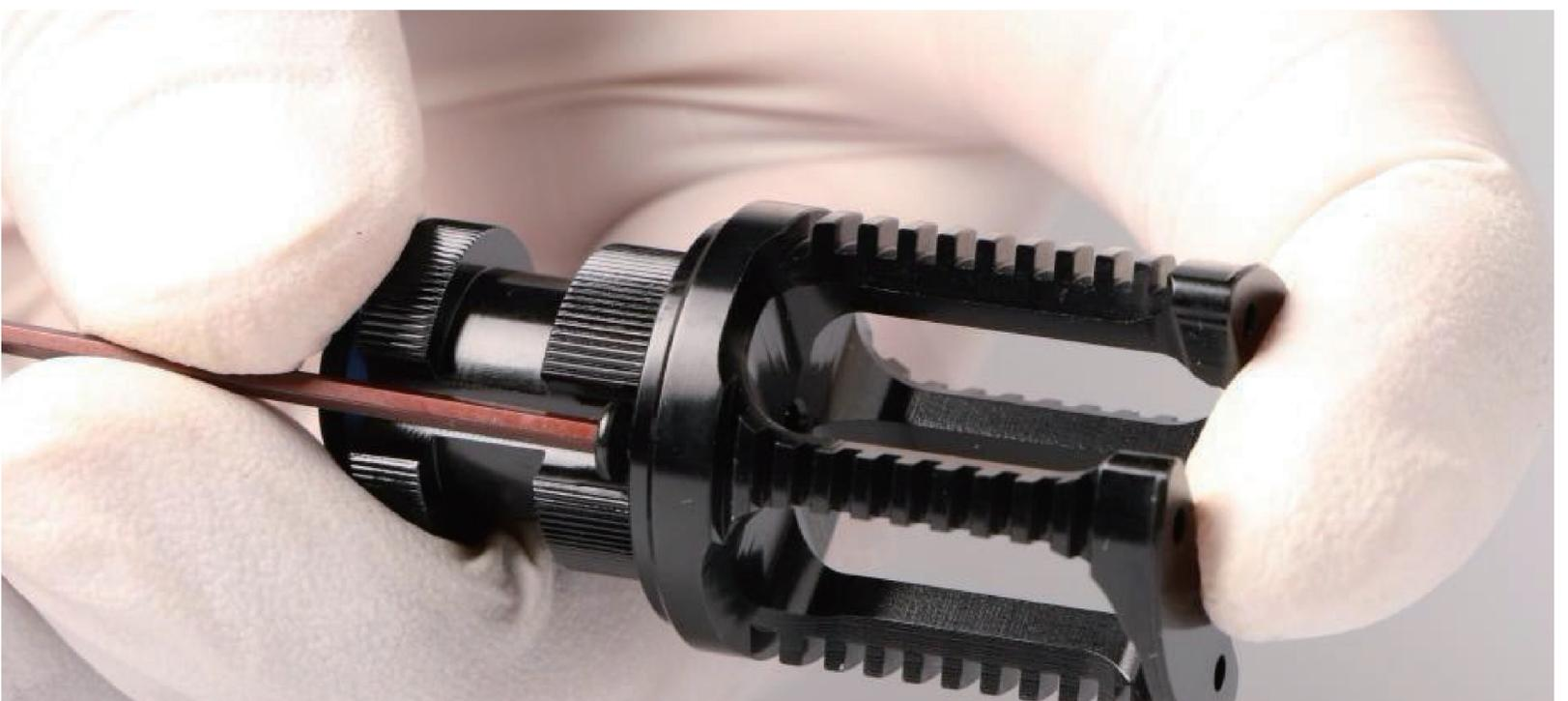
3. Tighten the heatbreak to the heatblock using the H7 wrench.
